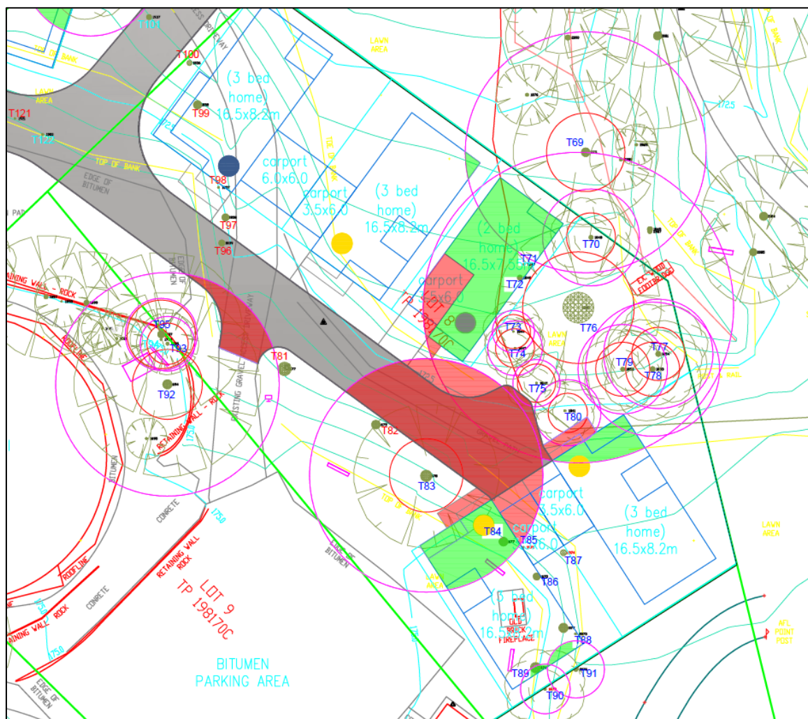
Figure 4: Works adjacent trees 69 – 100.
